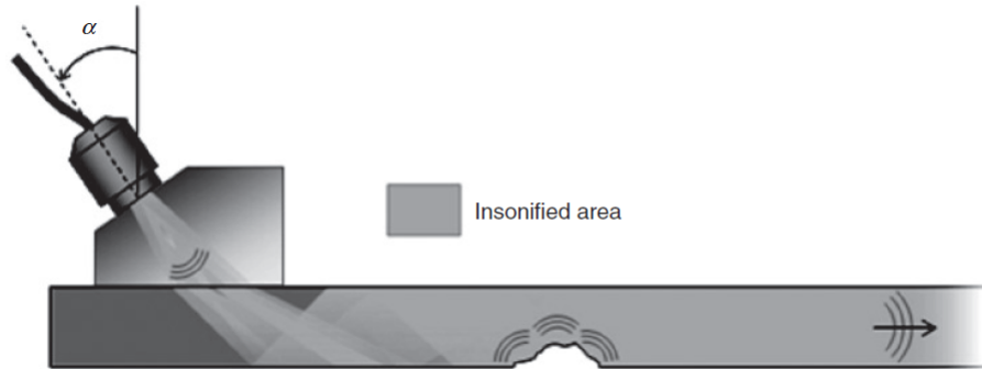
Figure 1.2 – Schematic of inspection of the entire area of a structure using guided waves [4].
