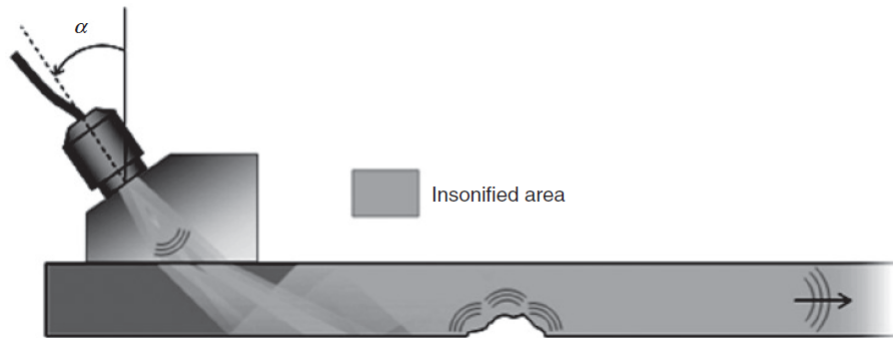
Figure 1.2 – Schematic of inspection of the entire area of a structure using guided waves [4].
