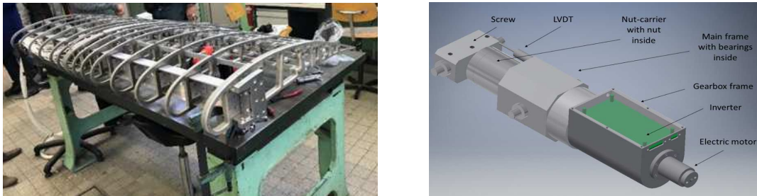
FIGURE 6.1: (left) : morphing flap assembling structure in the workshop laboratory of INPT/IMFT (right) : detailed CAD view of the EMA
