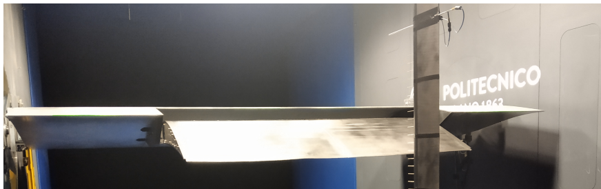
FIGURE 2.11: The LS prototype in POLIMI's wind tunnel involving the high-lift morphing flap constructed in the IMFT's workshop thanks to the structural design by (Bmegaptche et al. (2019)), in collaboration with LAPLACE (D. Harribey - J.F. Rouchon). Photo in the POLIM wind tunnel by courtesy of F. Auteri.
