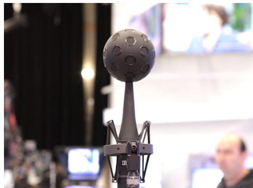
FIGURE 1.3 – Antenne de microphones Eigenmike de Mh Acoustics [Mh-Acoustics, 2013].
