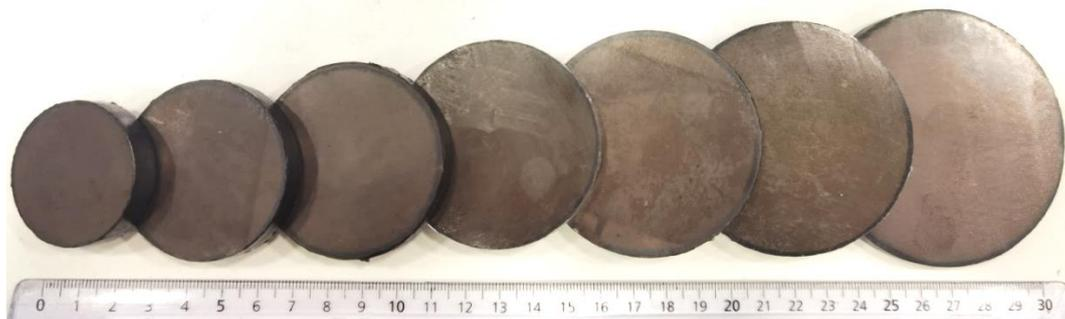
Fig.6-1: Photograph of ex-situ MgB<sub>2</sub> bulks with (A) various thickness and (B) various diameters.
