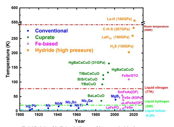
Fig.1-1 Evolution of the  $T_c$  since the discovery of the superconductivity phenomenon
