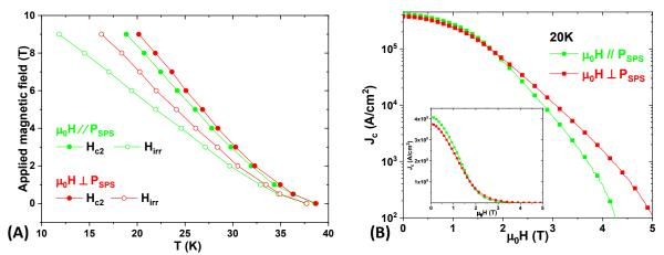
Fig.7-2: (A) Temperature dependence of  $H_{c2}$  and  $H_{irr}$  for different applied field directions. (B) Magnetic field dependence of the critical current density  $J_c$  at 20 K for different applied field directions. The inset shows the same curves on a linear scale.
