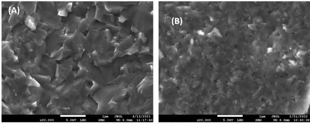
Fig.3-21: morphology of MgB<sub>2</sub> grains in (A) C1 and (B) C2 bulks
