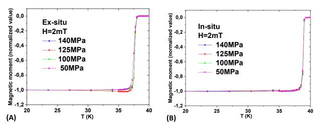
Fig.4-4: Normalized magnetic moment as a function of the temperature for (A) ex-situ and (B) in-situ bulks
