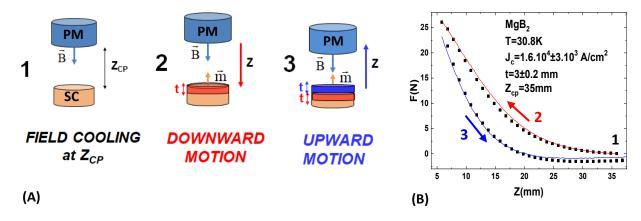
Fig.2-7: (A) Measurement procedure of the levitation force with the assumed locations of the currents interacting with the field of the magnet. (B) Levitation force hysteresis loop carried out between a 29.6 mm diameter  $MgB_2$  bulk and a 45 mm diameter magnet at 30 K after FC at  $Z_{cp}$  = 35 mm. The continuous lines show the values calculated with Eq.2.6-14. and the  $J_c$  and t values indicated in the figures [43].
