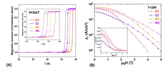
Fig.4-12: (A) Normalized magnetic moment of samples as a function of the temperature. (B) Magnetic field dependence of the critical current density  $J_c$  of samples at 20 K. The inset shows the same curves on a linear scale.
