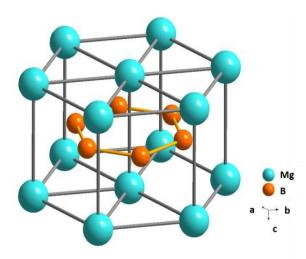
Fig.1-7 Crystal structure of MgB<sub>2</sub>
