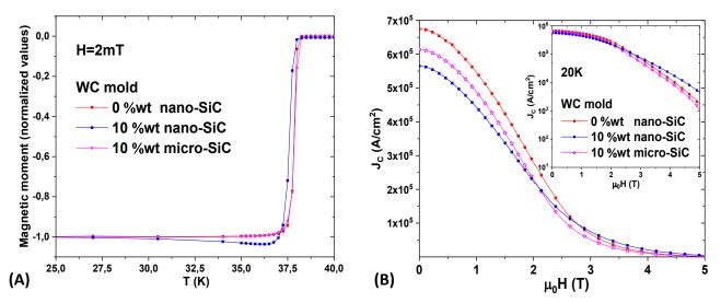
Fig.5-9: (A) Normalized magnetic moment as a function of the temperature for the 0 and 10 wt% micro- and nano-SiC doped samples sintered in WC molds. (B) Magnetic field dependence of the critical current density  $J_c$  at 20 K. The inset shows the same curves on a logarithmic scale.
