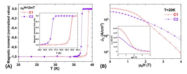
Fig.3-22: (A) Normalized magnetic moment as a function of the temperature. The inset shows the magnified onset of superconducting temperature. (B) Magnetic field dependence of the critical current density  $J_c$  at 20 K. The inset shows the same curves on a linear scale.
