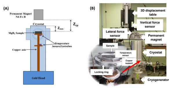
Fig.2-6 (A) Schema of the force measurements set-up. (B) picture of the cryocooler system and of the inside of cryostat
