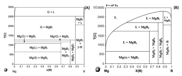
Fig.1-9 Mg-B binary phase diagrams at (A) atmospheric pressure and (B)100 MPa [63]
