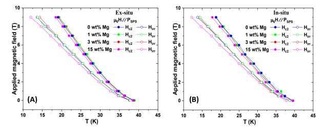
Fig.5-1:Temperature dependence of  $H_{c2}$  and  $H_{irr}$  for the (A) Ex-situ and (B) In-situ samples prepared by using graphite mold.  $H_{c2}$  and  $H_{irr}$  were determined from 90% and 10% of  $\rho_{40K}$ .
