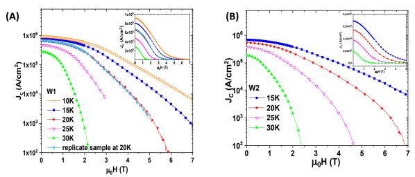
Fig.4-14: Magnetic field dependence of the critical current density  $J_c$  at various temperatures for (A) W1 and (B) W2 samples. The inset shows the same curves on a linear scale. Fig.4-13(A) also shows  $J_c(\mu_0 H)$  for a replicate sample at 20 K.
