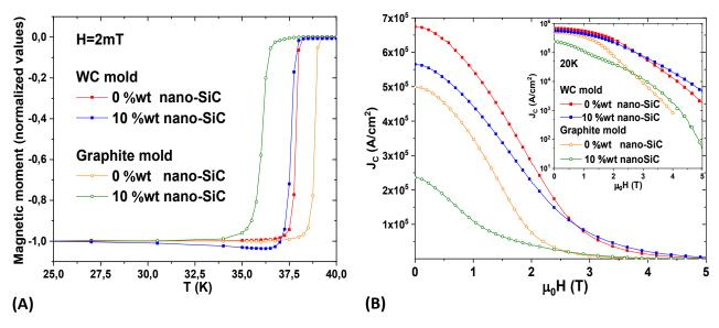
Fig.5-8: (A) Normalized magnetic moment as a function of the temperature for the 0 and 10 wt% nano-SiC doped samples sintered in different molds. (B) Magnetic field dependence of the critical current density  $J_c$  at 20 K. The inset shows the same curves on a logarithmic scale.
