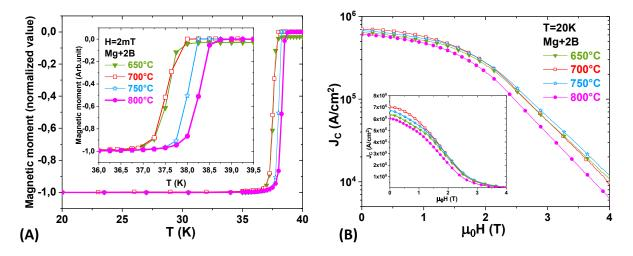
Fig.4-11: (A) Normalized magnetic moment vs. temperature for the samples processed at various temperatures. (B) Magnetic field dependence of the critical current density  $J_c$  at 20K for the samples processed at various temperatures. The inset shows the same curves on a linear scale.
