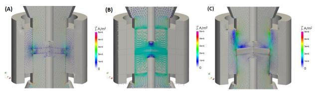
Fig.2-2 Schematic current flow in the case of: (A) conductive powder and die, (B) conductive powder and insulating die, (C) non-conductive powder and conductive die [87]
