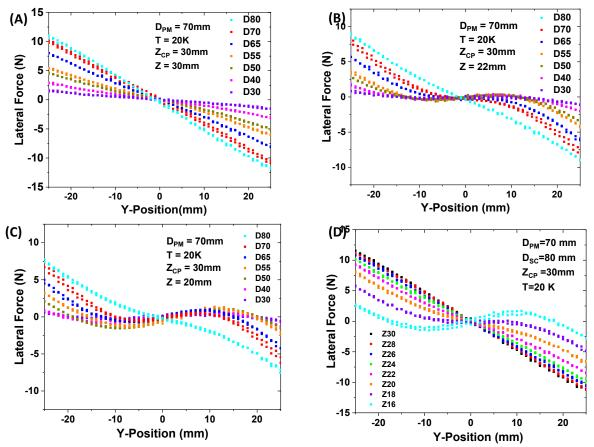
Fig.6-3: Lateral forces  $F_Y$  measured on MgB<sub>2</sub> discs with various diameters and the PM70 magnet at (A) Z = 30 mm, (B) Z = 22 mm and (C) Z = 20 mm after cooling down the MgB<sub>2</sub> discs at  $Z_{CP} = 30$  mm. (D) Lateral force  $F_Y$  measured with the 80 mm diameter MgB<sub>2</sub> disc at different magnet – disc separations, Z.
