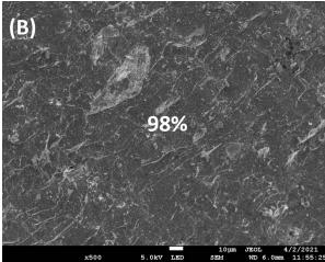
Fig.1-10 Microstructure of MgB<sub>2</sub> bulk fabricated by (A) CS [71] and by (B) SPS
