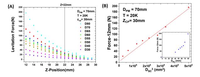
Fig.6-2: (A) Levitation force measurement carried out between a 70 mm diameter magnet and 10 mm thick MgB<sub>2</sub> bulks with various diameters at 20 K and  $Z_{cp}$ =30 mm. (B) Levitation force measured at  $Z_{min}$  = 12 mm as a function of  $D_{SC}$ <sup>3</sup>. The inset shows the levitation force as a function of  $D_{SC}$ .
