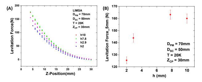
Fig.6-6: (A) Levitation forces carried out with various thick MgB<sub>2</sub> bulks at LIMSA. (B) Levitation force measured at  $Z_{min} = 5$  mm as a function of sample thickness, h.
