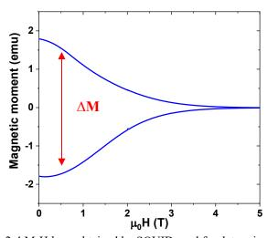
Fig.2-4 M-H loop obtained by SQUID used for determination  $J_c$
