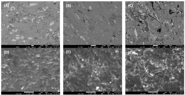
Fig.5-5: SEM micrographs of fractured surfaces of A) 10 wt% micro-SiC B) 10 wt% nano-SiC and C) 15 wt% nano-SiC doped samples sintered in WC mold and magnification of MgB<sub>2</sub> grains in the 10 wt% micro-SiC (D), 10 wt% nano-SiC (E) and 15 wt% nano-SiC (F) doped samples.
