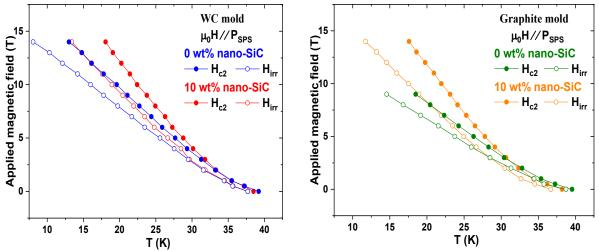
Fig. 5-7: Temperature dependence of  $H_{c2}$  and  $H_{irr}$  for the supples prepared in (A) WC mold and (B) Tc graphite mold.  $H_{c2}$  and  $H_{irr}$  were determined from 90% and 10% of  $\rho_{40K}$ .
