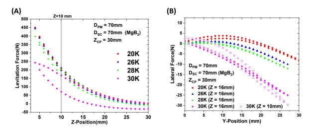
Fig.6-8: Comparison between 20-30 K of the (A) levitation forces and (B) lateral forces of 70 mm diameter and 10 mm thick MgB<sub>2</sub> disc after field cooling at 30 mm from the 70 mm diameter magnet.
