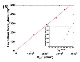
Fig.6-4: (A) Levitation forces carried out with various diameter MgB<sub>2</sub> bulks at LIMSA. (B) Levitation force measured at  $Z_{min} = 4$  mm with a 70 mm diameter magnet as a function of  $D_{SC}^{3}$ . The inset shows the levitation force as a function of  $D_{SC}$ .
