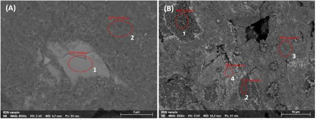
Fig.5-6: EDS analysis of the A) 10 wt% and B) 15 wt% nano-SiC doped samples sintered in WC molds
