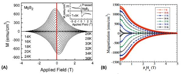
Fig.7-4: (A) *M-H* loops reported in [158] with a 2.18 x 2.76 x 1.88 mm<sup>3</sup> sample (B) *M-H* loops reported in [36] with a 1.5 x 1.5 x 0.5 mm<sup>3</sup> sample
