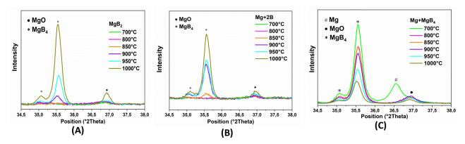
Fig.3-10: Local magnification of the MgO, MgB<sub>4</sub> and Mg peaks of A) MgB<sub>2</sub> B) Mg+2B and C) Mg+MgB<sub>4</sub> series sample sintered at 700-1000°C
