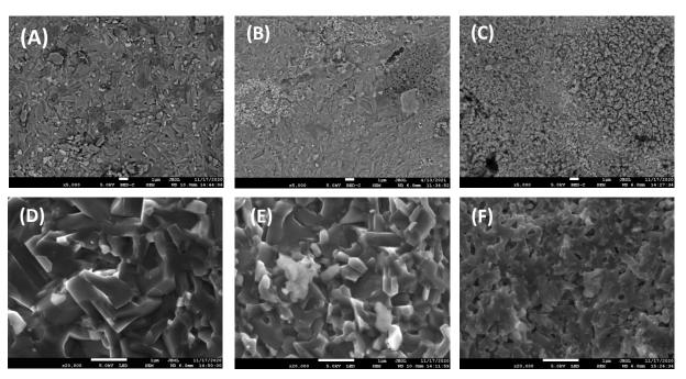
Fig.3-14: SEM micrographs of fractured surfaces of A) B1, B) B2 and C) B3 samples and magnification of MgB<sub>2</sub> grains in the D) B1, E) B2 and F) B3.
