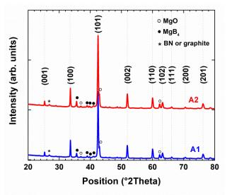
Fig.3-4 XRD analysis of MgB<sub>2</sub> bulks sintered with lot1 and lot2 ex-situ powders
