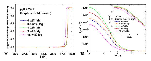
Fig.5-3: (A) Temperature dependence of the normalized magnetic moment of the batch 2 samples. (B) Magnetic field dependence of the critical current density J<sub>c</sub> at 20 K of the batch 2 samples. The inset shows the same curves on a logarithmic scale.
