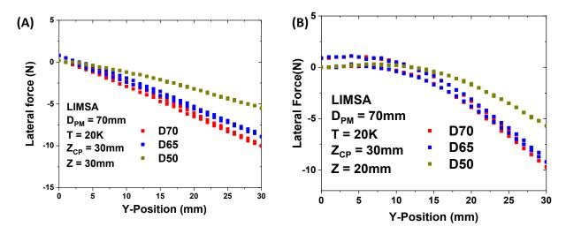
Fig.6-5: Lateral forces measured at (A) Z = 30 mm and (B) Z = 20 mm after cooling down the various diameter MgB<sub>2</sub> discs with various diameters at  $Z_{CP} = 30$  mm and 20 K.
