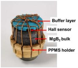
Fig.2-10 Picture of the PPMS sample holder with a MgB<sub>2</sub> bulk
