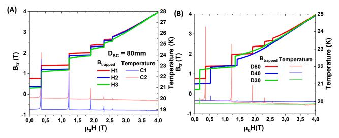
Fig.6-14: (A) Applied field dependence of trapped field and temperature for three positions of Hall probe and two positions of Cernox probe on the surface of the 80 mm diameter disc. (B) Applied field dependence of trapped field and temperature for three different diameter samples.
