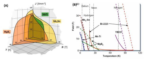
Fig.1-8 (A) Critical surfaces of MgB<sub>2</sub>, NbTi and Nb<sub>3</sub>Sn [59]. (B) Magnetic field vs. temperature phase diagram for several type II superconductors. The upper critical fields,  $H_{c2}$ , are indicated by dashed lines, the irreversibility fields,  $H_{irr}$ , by solid lines. [60]
