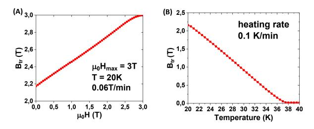
Fig.6-13: (A) Trapped field vs. applied magnetic field for the 20 mm diameter MgB<sub>2</sub> disc at 20 K. The applied field is 3 T, and the reduction rate is 0.06 T/min. (B) Trapped field vs. applied temperature with a 0.1 K/min heating rate.
