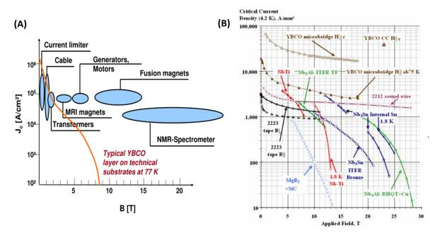
Fig.1-11: (A) Required properties for different power applications. (B) The critical current density of several type II superconductors dependence of applied field at 4.2 K [84]
