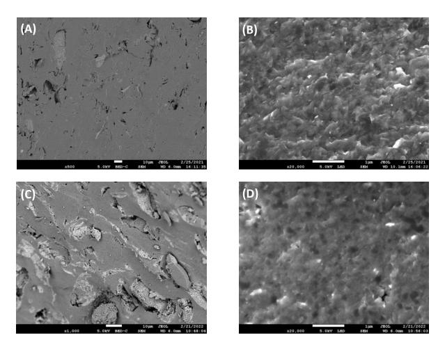
Fig.4-8: Chemical microstructure of (A) W1 and (C) W2 samples; High magnification SEM image of nano MgB<sub>2</sub> grains in (B) W1 and (D) W2 bulks.
