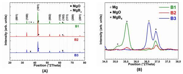
Fig.3-13: (A) XRD pattern of three bulks. (B) Local magnification of the MgO, MgB<sub>4</sub> and Mg peaks.
