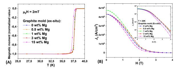
Fig.5-2: (A) Temperature dependence of the normalized magnetic moment of the samples of batch 1. (B) Magnetic field dependence of the critical current density  $J_c$  at 20 K of the samples of batch 1. The inset shows the same curves on a logarithmic scale.
