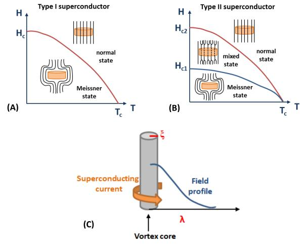
Fig.1-5 Phase diagram H=f(T) of (A) type I and (B) type II superconductor. (C) Schematic of a vortex produced by magnetic flux penetration in the mixed state of a type II superconductor
