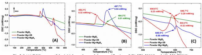
Fig.3-8 (A) DSC curves of the initial powders and the magnification of (B) 370-590°C and (C) 550-730°C.
