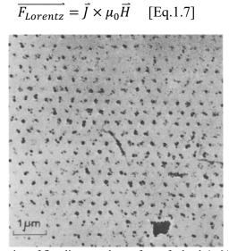
Fig.1-6 "Perfect" triangular lattice of flux lines on the surface of a lead-4at%indium rod at 1.1 K. [30]
