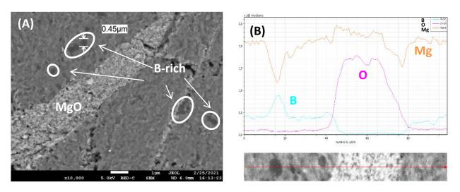
Fig.4-9: (A) SEM micrograph of sample W1 showing the unreacted boron and MgO regions in the MgB<sub>2</sub> matrix. (B) EDS red line region scan curves of B (cyan line), O (magenta line) and Mg (orange line).
