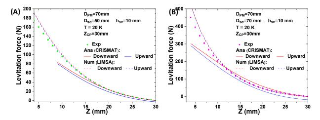
Fig.6-11: Force cycles of (A) the 50 mm and (B) the 70 mm diameter MgB<sub>2</sub> bulk measured at LIMSA. The continuous lines show the values calculated with the CRISMAT analytical model. The dashed lines show the values estimated with the numerical model used at LIMSA.
