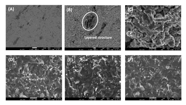
Fig.4-2: (A) SEM micrographs detected by back-scattered electrons of ex-situ sample sintered at 140 MPa and (B) the local magnification. (C)-(F) are the topographic view of MgB<sub>2</sub> grains detected by the secondary electrons in ex-situ samples sintered under 50-140 MPa, respectively
