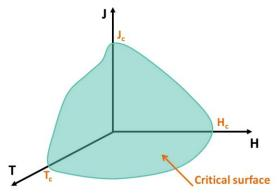
Fig.1-2 Relationship between  $T_c$ ,  $J_c$  and  $H_c$  in superconducting materials
