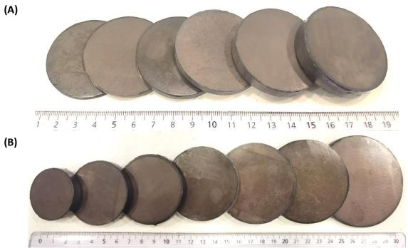
Fig.6-1: Photograph of ex-situ MgB<sub>2</sub> bulks with (A) various thickness and (B) various diameters.
