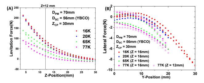
Fig.6-9: Comparison between 16 K and 77 K of the levitation forces (A) and of the lateral forces (B) of a 56 mm diameter and 16 mm thick YBaCuO disc after field cooling at 30 mm from the 70 mm diameter magnet.
