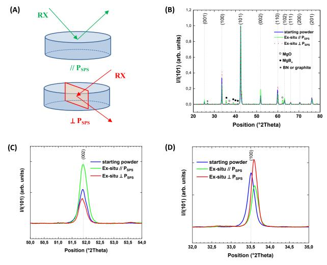
Fig.7-1: (A) The indication of the XRD measurements direction for the sintered  $MgB_2$  disc. (B) XRD patterns of the initial powder and the sintered bulk obtained on different surfaces. The intensity is normalized by the peak (101), which is the most intense peak for a randomly oriented sample. (C) and (D) shows the magnified results of (002) and (100) peak, respectively.
