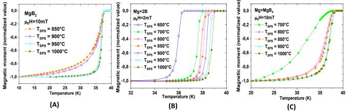
Fig.3-11: Normalized magnetic moment - temperature curves of A) MgB<sub>2</sub>, B) Mg+2B and C) Mg+MgB<sub>4</sub> series.
