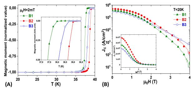
Fig.3-16: (A) Normalized magnetic moment of samples B1, B2 and B3 as a function of the temperature. The inset shows the onset of superconducting temperature. (B) Magnetic field dependence of the critical current density  $J_c$  at 20 K. The inset shows the same curves on a linear scale.
