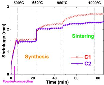
Fig.3-19: Displacement of piston vs. sintering time curves.
