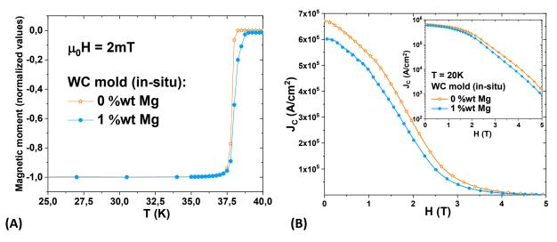
Fig.5-4: (A) Temperature dependence of the normalized magnetic moment of the samples of batch 3; (B) Magnetic field dependence of the critical current density  $J_c$  at 20 K of the samples of batch 3. The inset shows the same curves on a logarithmic scale.
