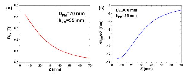
Fig.6-10: Field (A) and field gradient (B) along the axis of the NdFeB magnet used during the measurements.
