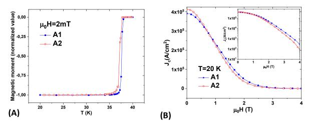
Fig.3-6 (A) Normalized magnetic moment as a function of the temperature. (B) Magnetic field dependence of the critical current density  $J_c$  at 20 K. The inset shows the same curves on a logarithmic scale.
