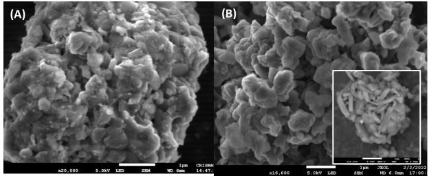
Fig.3-2 SEM micrographs of ex-situ powders supplied by (A) PAVEZYUM, Turkey, lot1 and (B) abcr, Germany, lot2. The inset in Fig.3-2(B) shows the platy structure of MgB<sub>2</sub> grains present in lot 2 powder.
