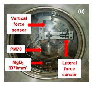
Fig.2-9 Pictures of the cryocooler system at LIMSA (A) and of the inside of cryostat (B)
