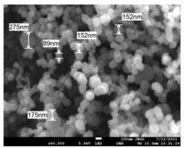
Fig.3-7 SEM micrographs of amorphous nano boron.
