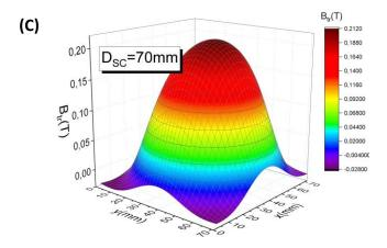
Fig.6-12: Magnetic mapping of (A) 20, (B) 40 and (C) 70mm diameter MgB<sub>2</sub> discs.
