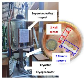
Fig.2-11 Picture of the device used for measuring the field trapped by superconducting discs at Institute Néel.
