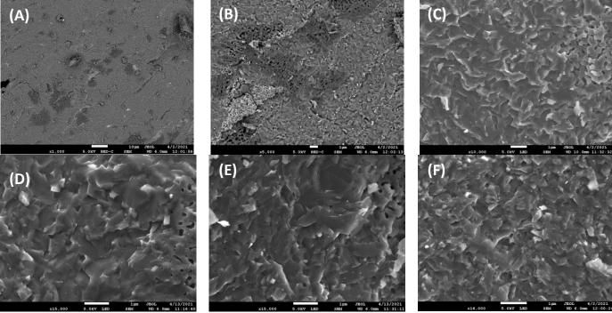
Fig.4-3: (A) SEM micrographs detected by back-scattered electrons of in-situ sample sintered at 140 MPa and (B) the local magnification. (C)-(F) are the topographic view of MgB<sub>2</sub> grains detected by the secondary electrons in in-situ samples sintered under 50-140 MPa, respectively
