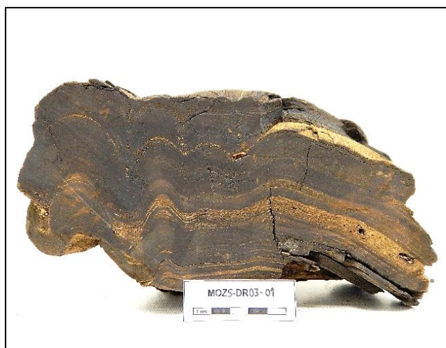
Figure 1.7. Fe-Mn crust MOZ5-DR03-01 of which different periods are visible thanks to the laminations. PAMELA-MOZ5 (Moulin, Evain, 2016).
