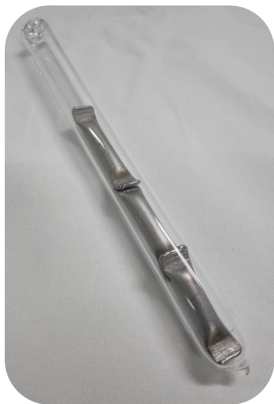
FIGURE II.3 – Tubes de niobium scellés en tube de silice.
