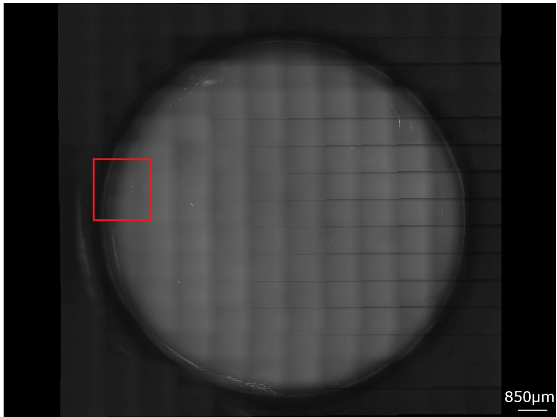
FIGURE 4.21: Sensofar picture after the third thermal treatment, bright field. There is no difference in contrast between the former adherent and non-adherent parts. The red box identifies the reference for Figure 4.22.
