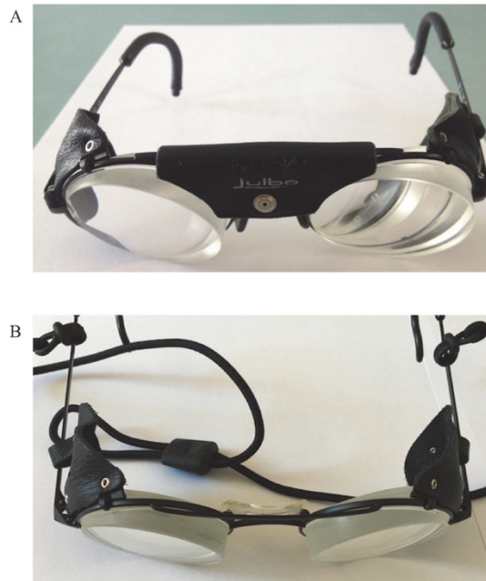
A, a pair of prismatic glasses with an optical deviation of 10 degrees towards to the right side; B, a pair of sham glasses with a neutral optical deviation.
