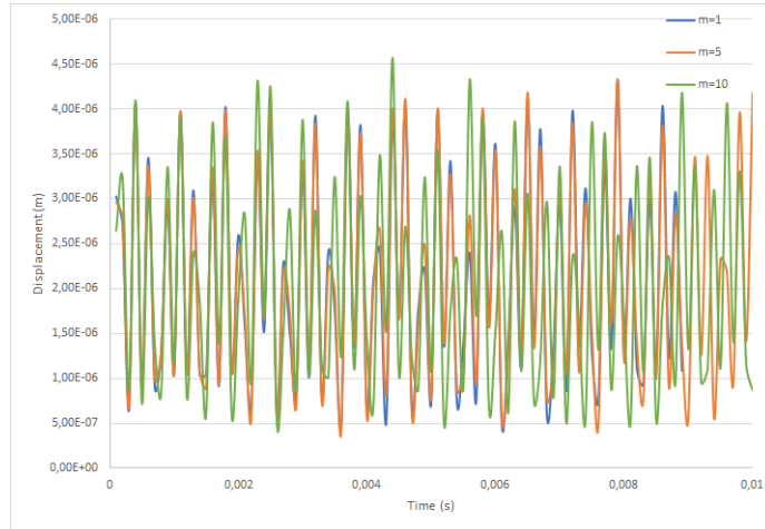
FIGURE 3.15: Displacements of the point of interest according to the time, with different time scale ratio and conforming meshes
