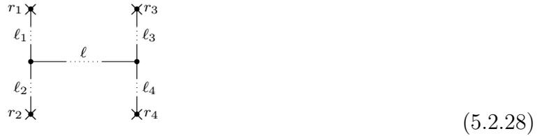
where upper left, lower left, upper right and lower right vertical branches have respective lengths  $\ell_1, \ell_2, \ell_3, \ell_4$ , while the connecting horizontal branch has length  $\ell$ . Up to factors of  $\lambda_{(r_{id})}$  from summing out the loops not separating the marked points, we get the weight
