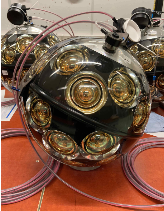
Figure 4.1: Digital optical module (DOM) at the KM3NeT construction site at NIKHEF, Amsterdam. The multi-PMT design yields a high photocathode area and allows for better trigger conditions and event reconstruction.
