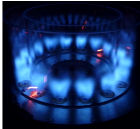
Figure 1.5: Annular combustor MICCA designed at the EM2C laboratory, equipped with 16 swirled fuel injectors and operated with propane/air mixtures. Image taken from Bourgouin et al. (2013) .
