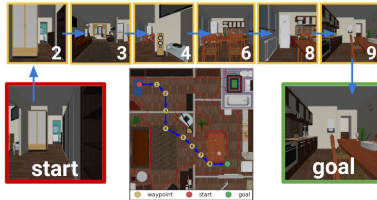
Figure 2.32: Steps of Search on the Replay buffer. When provided with an initial state and a goal state, their system finds a sequence of intermediate waypoints. A lower level agent can follow these waypoints to navigate to the goal. Figure from (Eysenbach et al. 2019a).
