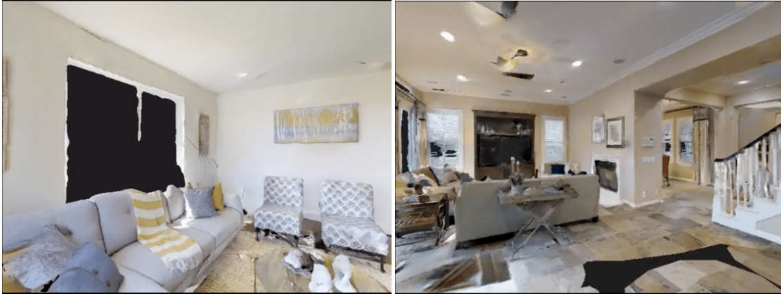
Figure 2.24: Example environments in the Habitat simulator , shown are renderings from virtual monocular cameras in two homes. There are artifacts in the 3D reconstruction due to interference from external intra-red light sources and from occlusions, nevertheless the reconstructions are of relatively high quality. (Savva et al. 2019a).
