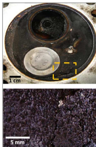
Figure 7: Enlarged image of cylinder-head deposits [38].
