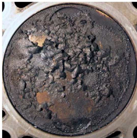
Figure 27: Piston with deposits flaking [80].
