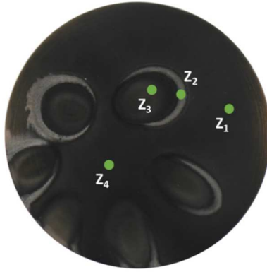
Figure 77 : Location of the Raman measurement zones Z_n (green dots) for the late injection experiment.
