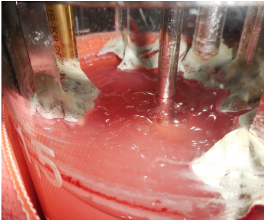
Figure 3 (a): surface of the liquid culture of T. albobiverticillius without bubbling (50 % DO 2 ), with an agitation of 200 rpm (day 7)
