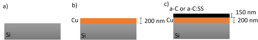
Figure 4.2: Schematic representation of the sandwich-like samples using a) Silicon as substrate; b) 200 nm of copper films were deposited using DCMS, and lastly, c) carbon-based films were deposited over the Si/Cu films.
