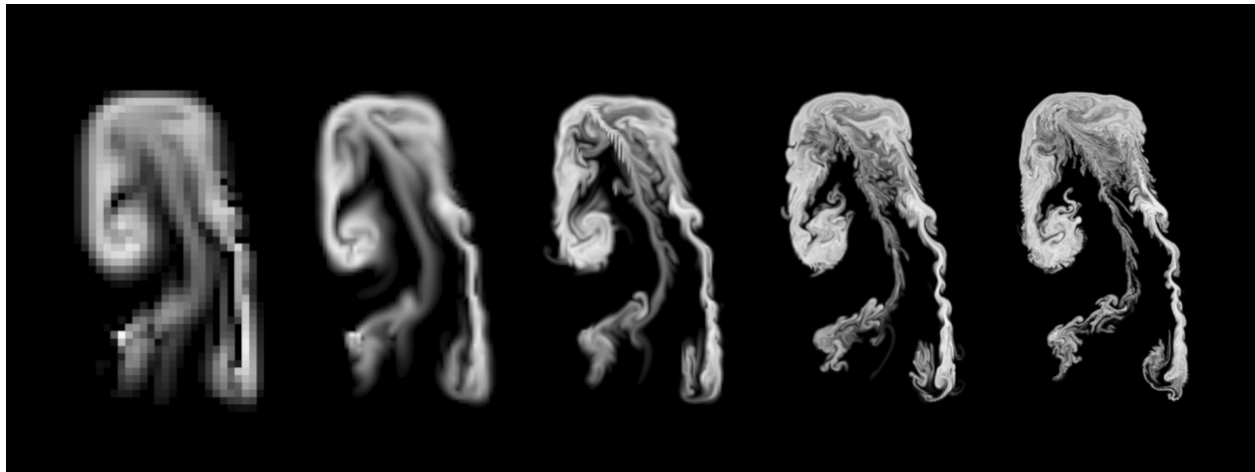
Fig. 4.4.1. 2D rising plume. Left to right: Guide ( 32 \times 48 ), tracked 2\times , 4\times , 8\times , and 16\times . The larger the upresolution factor, the finer the added simulated details.
