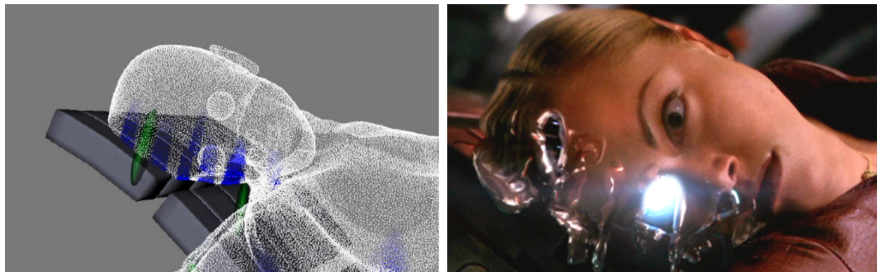
Fig. 2.2.16. Control applied on a metallic liquid simulation using the method of Rasmussen et al. [95]. Left: Control particles in white apply hard velocity constraints. Control particles in blue apply soft velocity constraints, leading to an effect of melting and flowing. Green regions represent CSG (Constructive Solid Geometry) level set liquid erasers. Right: Final rendering of the scene.
