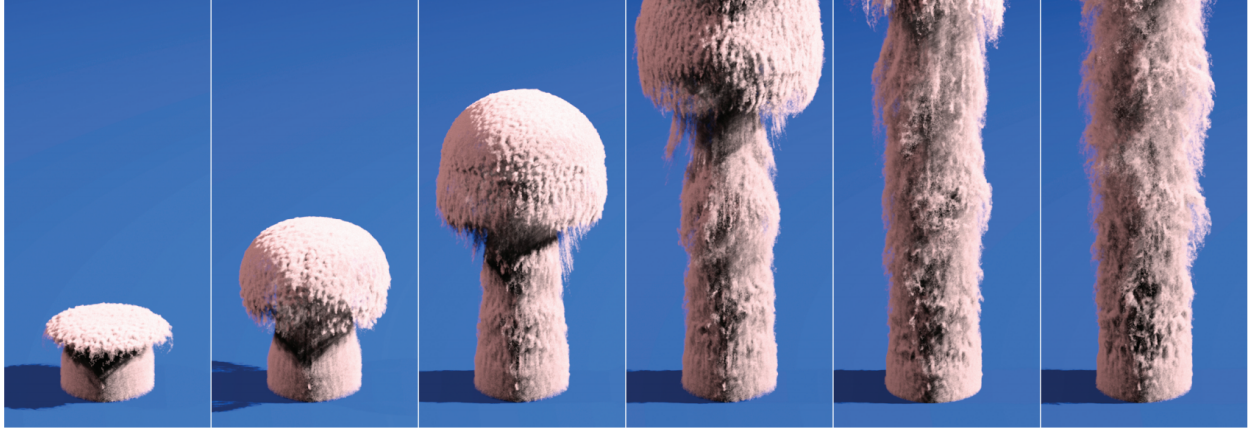
Fig. 2.5.5. A 12800 \times 25600 \times 12800 generated by adding eight turbulence spectral bands to an input 50 \times 100 \times 50 smoke simulation using the method of Kim et al. [60].
