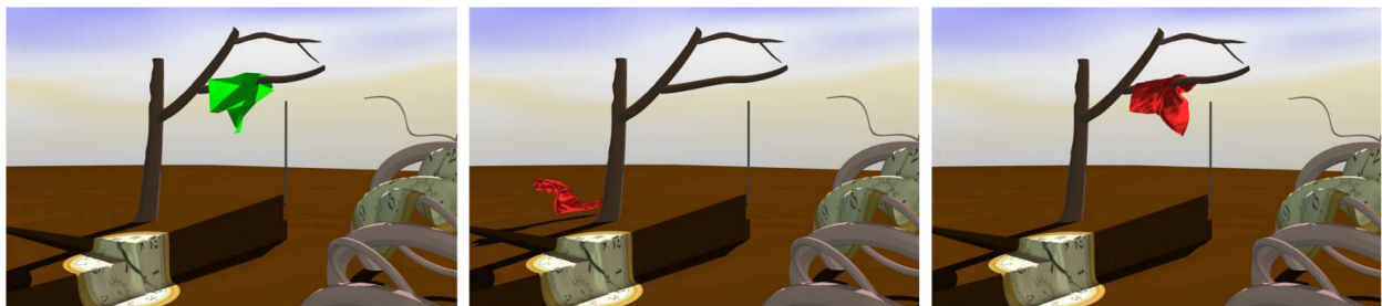
Fig. 2.5.1. Example of tracking using the TRACKS [12] framework. Left: Low-resolution guide simulation. Center: High-resolution free simulation, generated with the same initial conditions than the guide simulation. Note that the simulation does not exhibit the same behavior than the guide. Right: High-resolution tracked simulation. The high-resolution simulated piece of cloth closely follows the guide, but is enhanced with small-scale physically simulated details.
