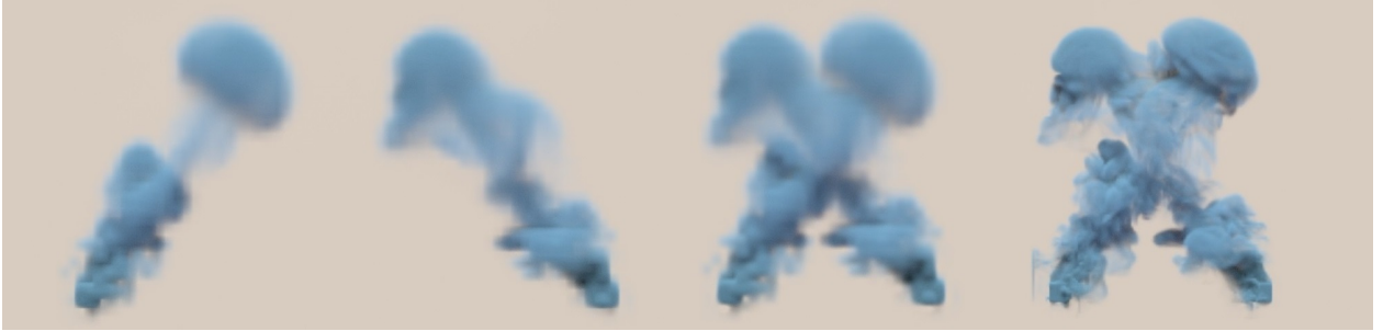
Fig. 4.4.11. Tracking the combination of two rising plumes. From left to right: A first low-resolution plume of smoke rising towards the top right corner, a second plume of smoke rising towards the top left corner, the result of the combination (by density summation) of the two previous simulations, and a tracked simulation generated using our method.
