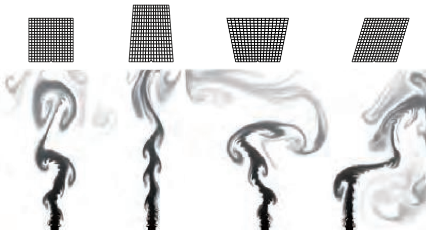
Fig. 2.2.21. Controlled smoke simulations in 2D from Pan and Manocha [87]. A simulation is performed on a regular uniform grid (leftmost image). Simulations are generated using the same initial conditions but with three deformed grids.
