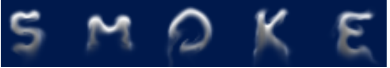
Fig. 2.2.1. Five separate 2D simulations ( 50 \times 50 , computation time: \sim 2 - 5h ) generated using the method of Treuille et al. [125] and forming each letter of the word “SMOKE”.
