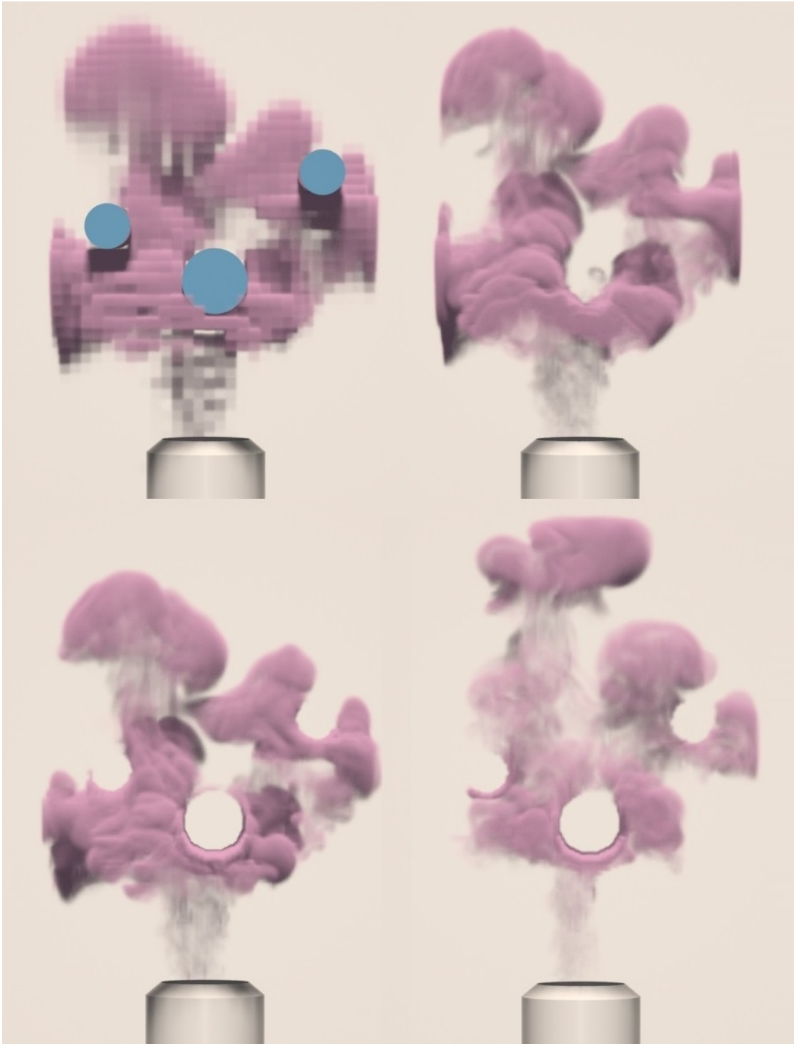
Fig. 4.4.8. Tracking a low-resolution smoke interacting with cylinders (not displayed). Top left: Guide. Top right: Tracked simulations using our method without boundary conditions enforced. Bottom left: Tracked simulations using our method with boundary conditions enforced. Bottom right: Free with the cylinders, exhibiting a much different smoke distribution.
