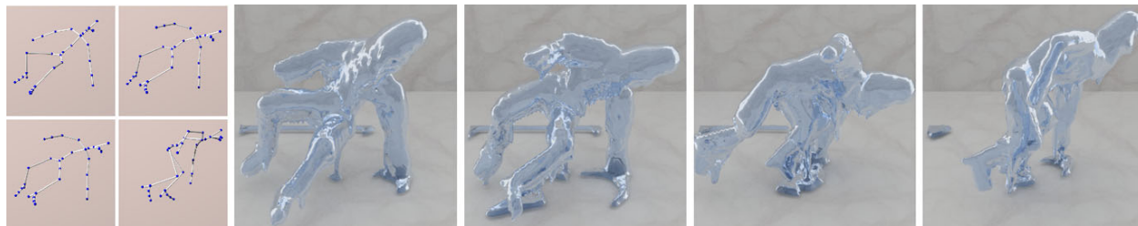
Fig. 2.2.10. Liquid controlled to match an animated skeleton using the method of Zhang et al. [139]. The four leftmost images show poses of a skeleton at four different times. The remaining four images represent the liquid surface controlled using the skeleton, at times corresponding to these poses.
