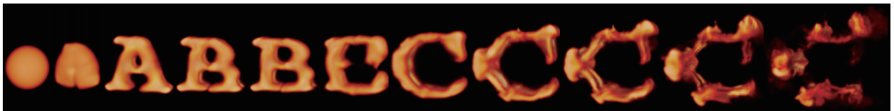
Fig. 2.2.3. Smoke simulation in 3D ( 64 \times 64 \times 64 , 150 frames, computation time: \sim 26h ) generated using the method of Pan et al. [88]. The target changes during the simulation, and goes from letter “A” to “B” to “C”.
