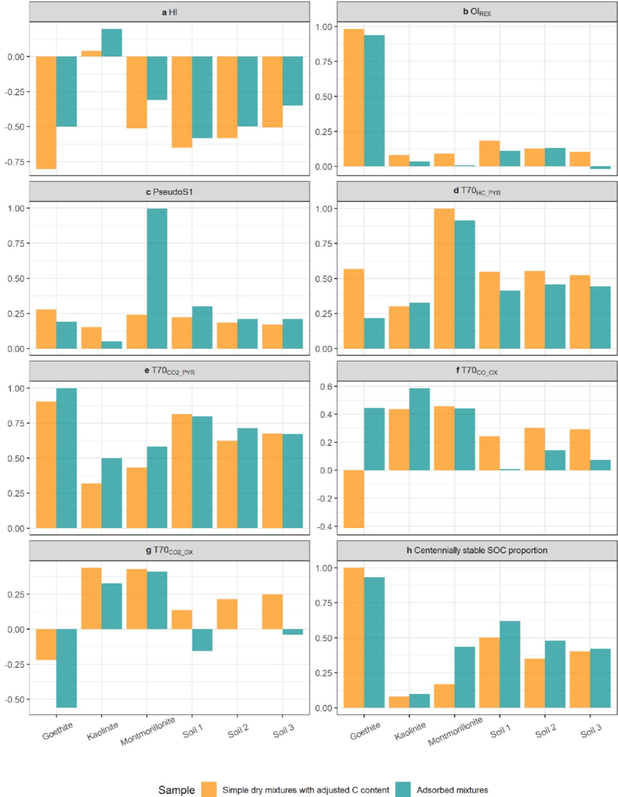
Figure 36: Effect of organo-mineral interactions on Rock-Eval® parameters. Orange bars represent dry mixtures of bovine serum albumin with different minerals, whereas blue bars represent adsorbed mixtures of the same compound. Parameter values shown here present the change relative to the pure compound signal (sand) normalized by the range of each parameter (see Sect. 2.3.6).
