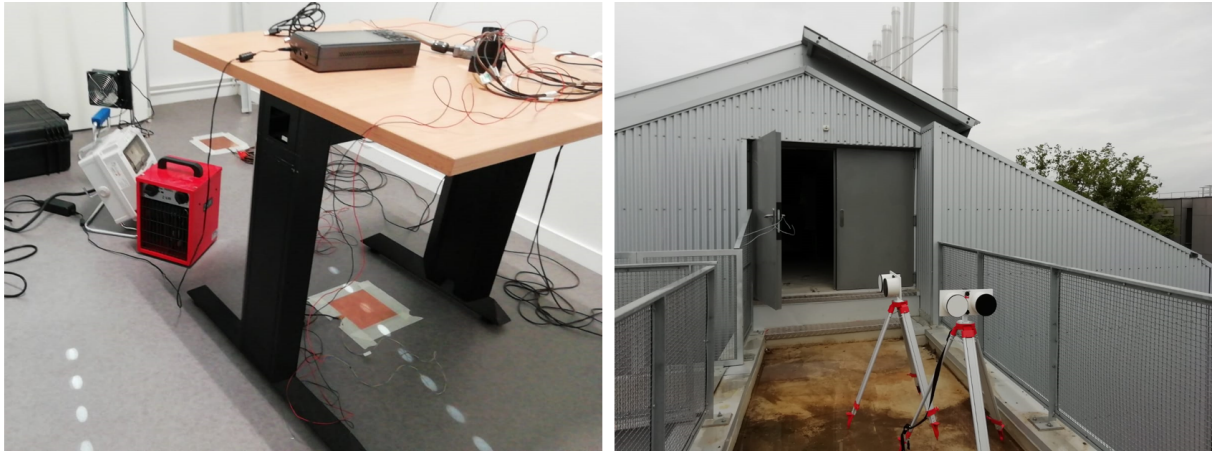
Figure 6.44 – SEREINE Heating module placed in the tested office (left), SENS sensors placed outside the building in the footbridge in front of the entrance of the unheated space (right).
