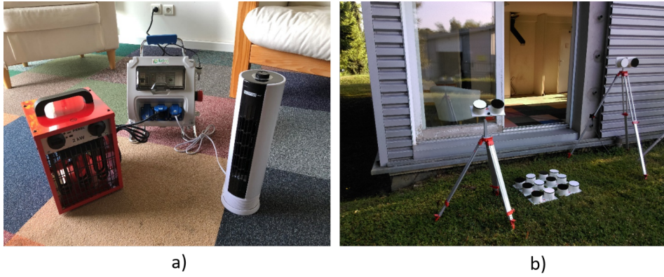
Figure 3.7 – a) ISABELE heating module, b) SENS sensors [176]
