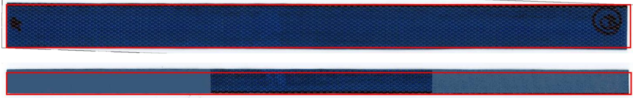
Fig. 2. 13. Example of difference between theoretical (red rectangle) and real prepreg dimensions after cut stage for ply#2
