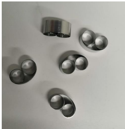
Fig. 3. Springs for fixing the samples in the resin
