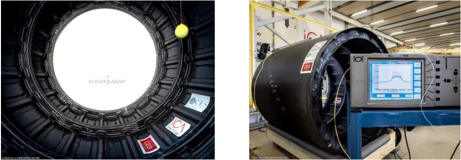
Fig. 1. 15. Manufactured prototype of composite fuselage from BLAST project [42] (scale 1/3)
