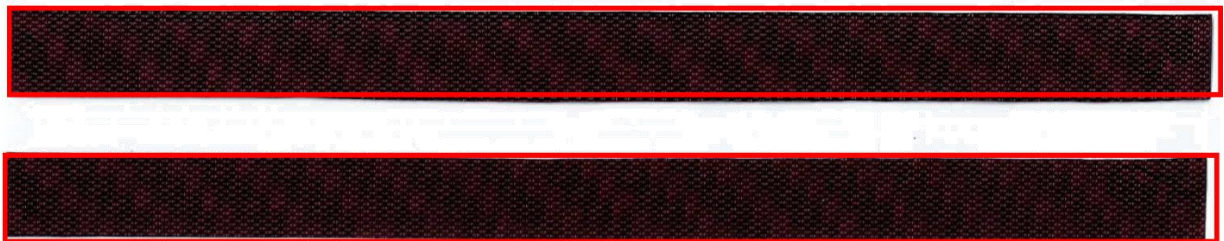
Fig. 2. 12. Example of difference between theoretical (red rectangle) and real prepreg dimensions after cut process for ply#4
