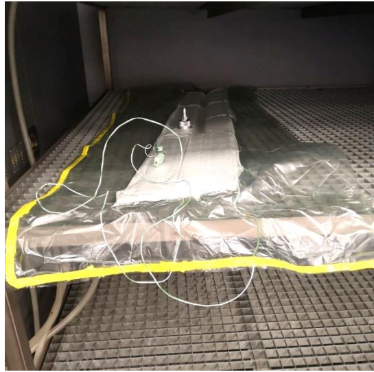
Fig. 2. 9. Structure covered with vacuum bag and prepared for polymerisation in the oven
