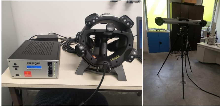
Fig. 2. 18. Scanning device used for 3D scan, the hand-held on the left and the scanner on the right
