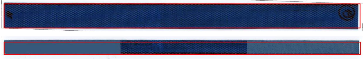
Fig. 2. 13. Example of difference between theoretical (red rectangle) and real prepreg dimensions after cut stage for ply#2
