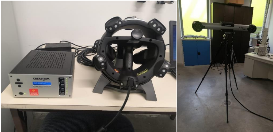
Fig. 2. 18. Scanning device used for 3D scan, the hand-held on the left and the scanner on the right
