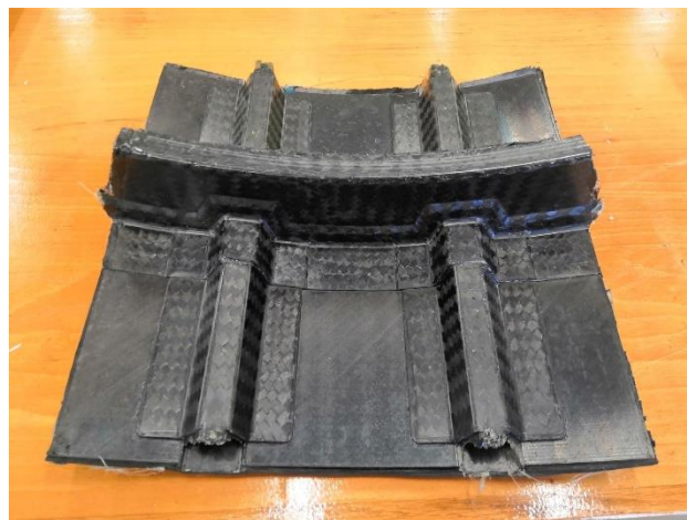
Fig. 8. Composite fuselage part obtained after curing
