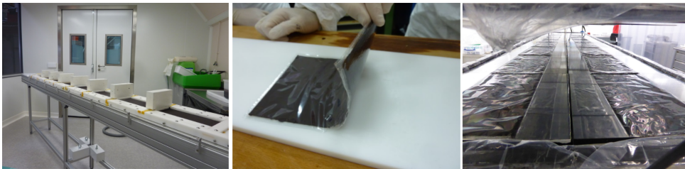
Figure 2.3 – To the left : The mylar pads that the selenium+PVA was poured on. In the middle : Selenium LAPP pad after it has dried, the edges are mylar. To the right : Selenium LAPP source foils after having 8 pads attached together.
