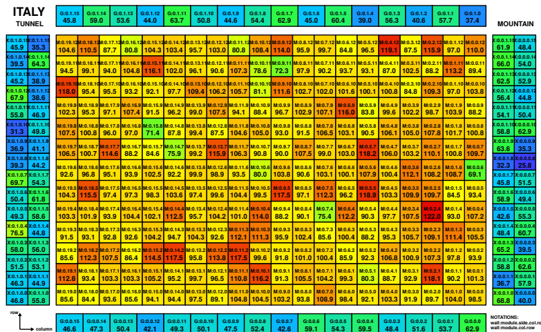
Figure 3.1 – Example map of the Italian calorimeter main wall. Filled with random numbers.
