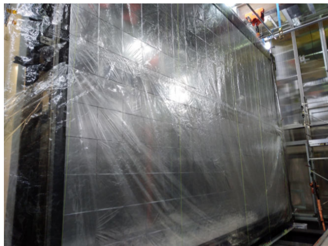
Figure 2.17 – A calorimeter wall covered with radio-pure nylon film. To avoid Radon diffusion from the calorimeter towards the tracker gas
