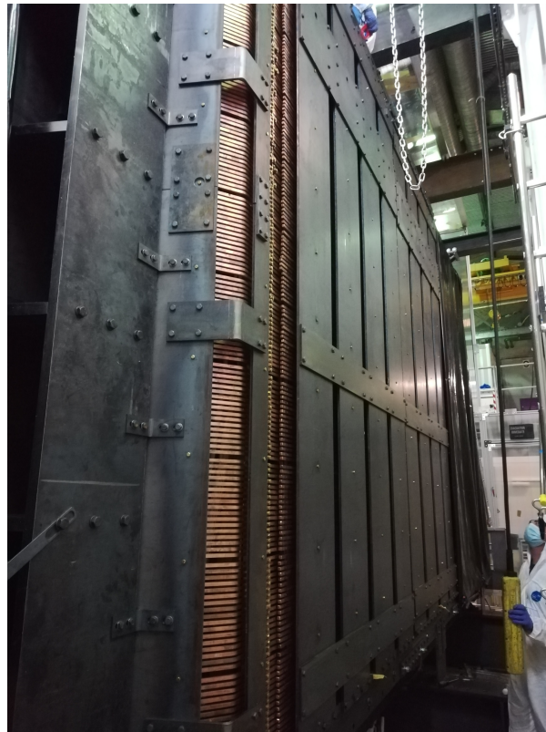
Figure 2.18 – Magnetic coil installed at the experiment site. The coil surrounds the detector. One side is shown in the figure.
