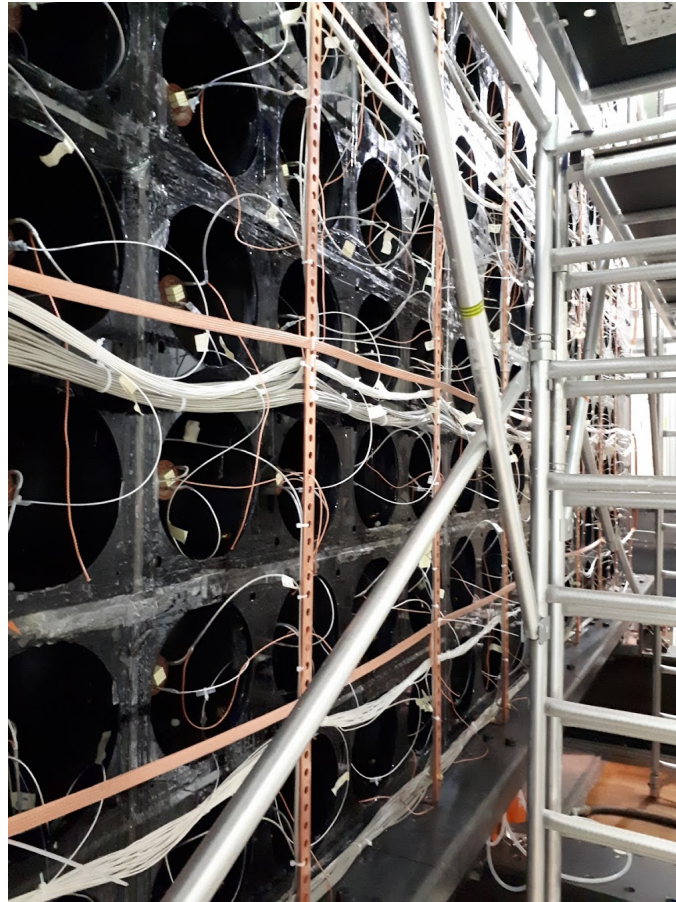
Figure 2.9 – Side view of a main calorimeter wall. Visible are the optical fibers, electric cables and signal cables, which deliver the high voltage and retrieve the PMT signals.
