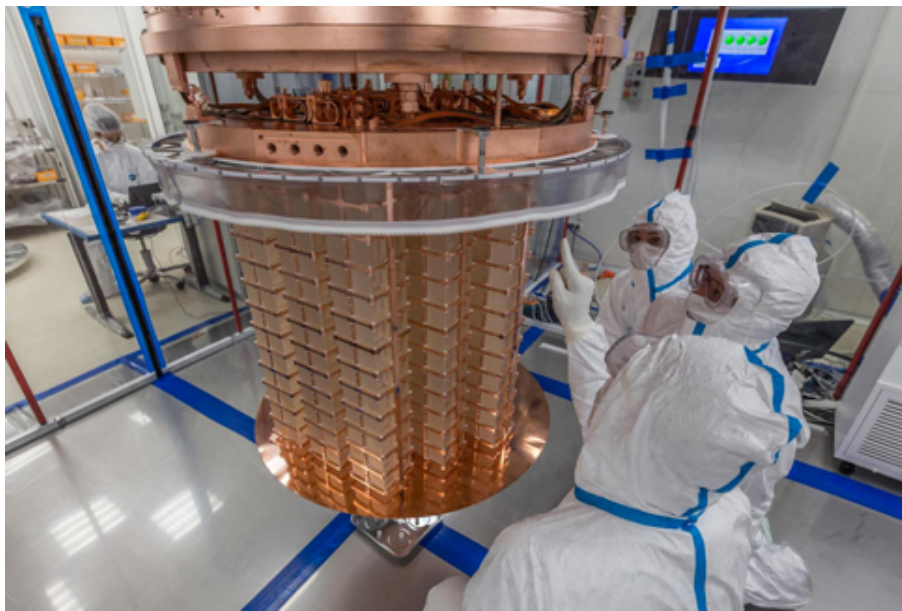
Figure 1.18 – The CUORE detector with the crystal towers. To avoid any contamination of the crystals, the construction of the detector has to be performed in clean rooms.
