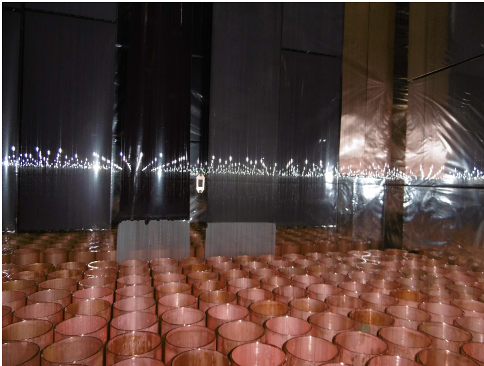
Figure 2.8 – The tracker cathode cells, along with the anode wires with light reflected on them. The source foils can also be seen (grey, middle).
