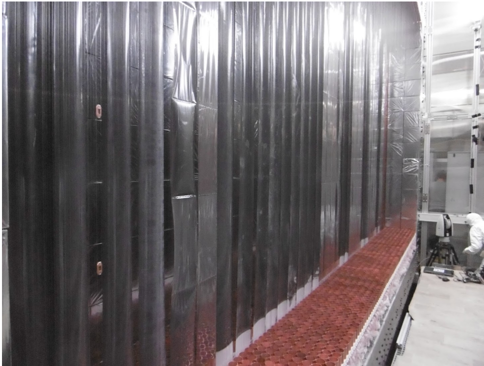
Figure 2.4 – Picture of the source foils (in dark grey) hanging inside the SuperNEMO demonstrator. One can spot the two types of foils : the LAPP (with foils pads attached together) and the ITEP foils.
