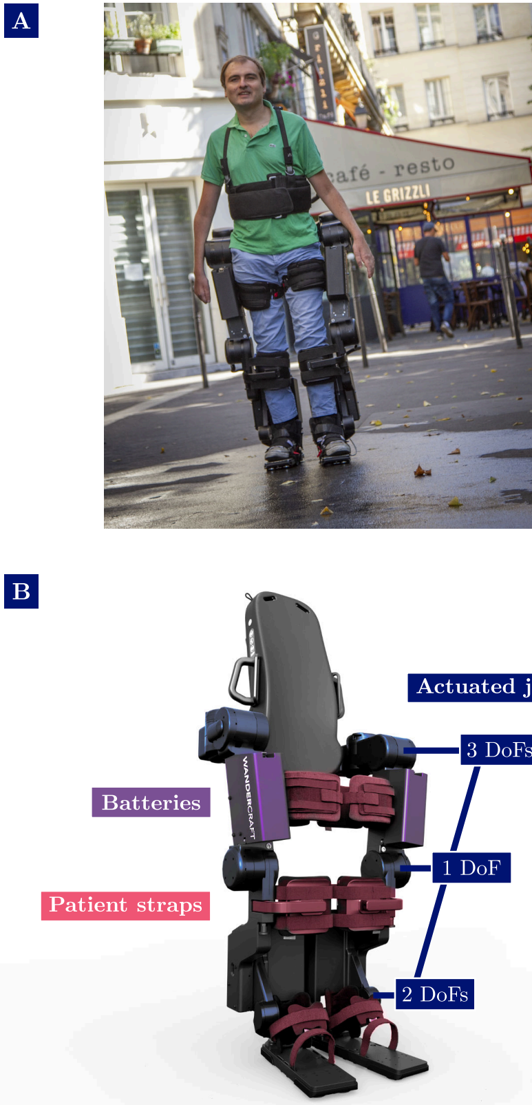
FIGURE 2.1: A. A patient walking in the Atalante exoskeleton during an outside tetherless test. B. The Atalante exoskeleton and some of its features. The blue parts indicate the joint actuators. The pink parts indicate the patient straps. The purple parts indicate the two batteries.
