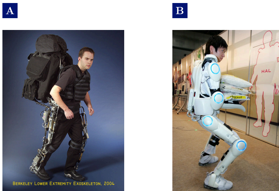
FIGURE 1.3: Augmentation exoskeletons for military and industrial applications: A. BLEEX by the Berkeley Robotics & Human Engineering Laboratory. B. HAL by Cyberdyne.
