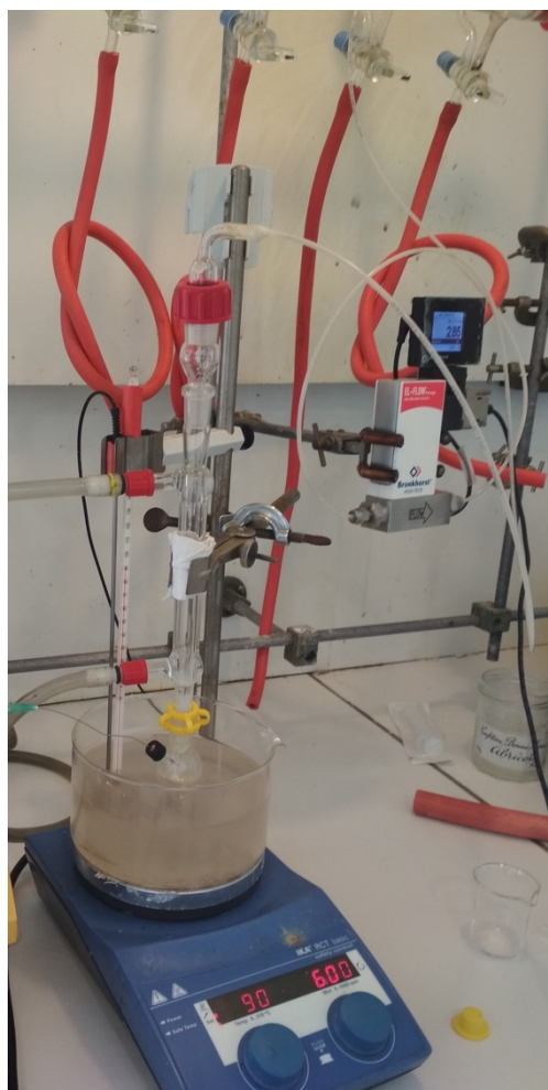
Figure IV - 2 - 2: Experimental set-up for FA dehydrogenation.
