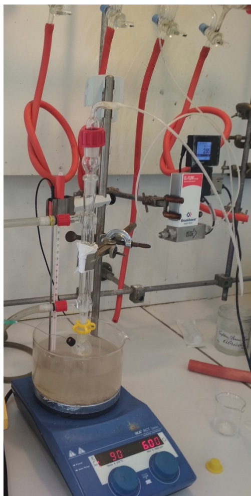
Figure IV - 2 - 2: Experimental set-up for FA dehydrogenation.
