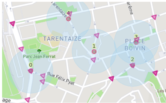
Figure 8.1: A sample AV-OLRA problem instance, with demand sources (triangles) and taxis (circles) with their respective communication ranges (in blue).
