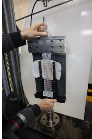
Figure 4.43: Mounting the pull-out device in the tensile machine
