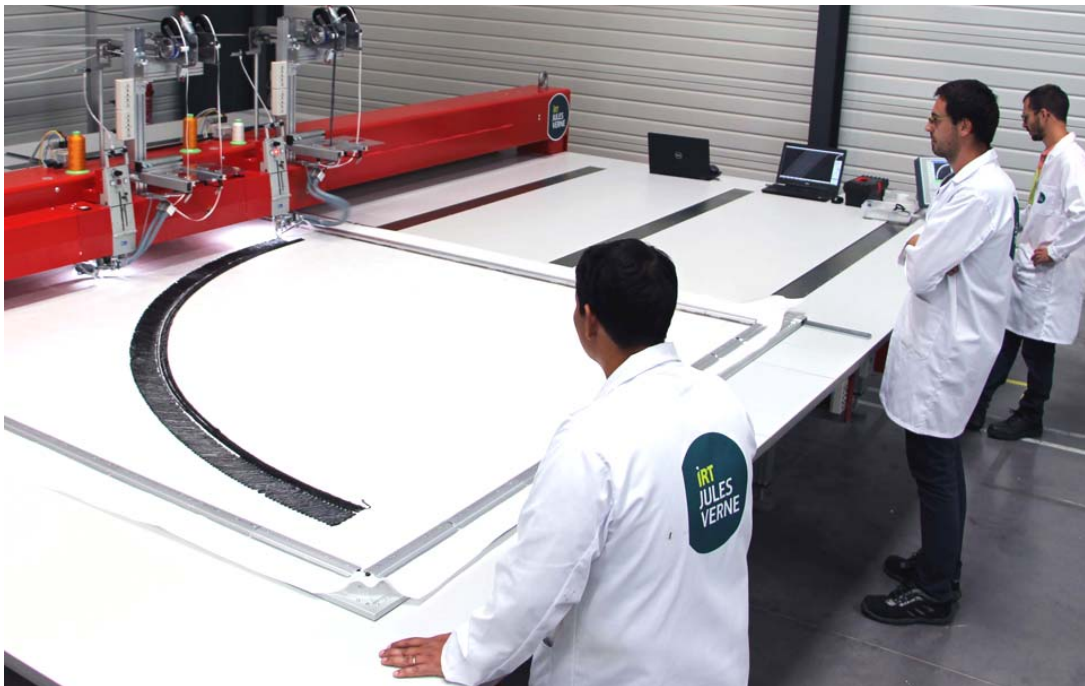
Figure 3.2: TFP machine used at IRT Jules Verne (TFP ZSK © CMCW 0200-900D-2500)
