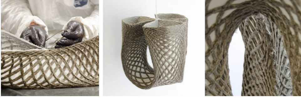
Figure 1.45: Stitching of the legs (a) and forming of preform under self-weight (b). Closeup photography of the stitched legs after curing (c) (Rihaczek et al., 2020)
