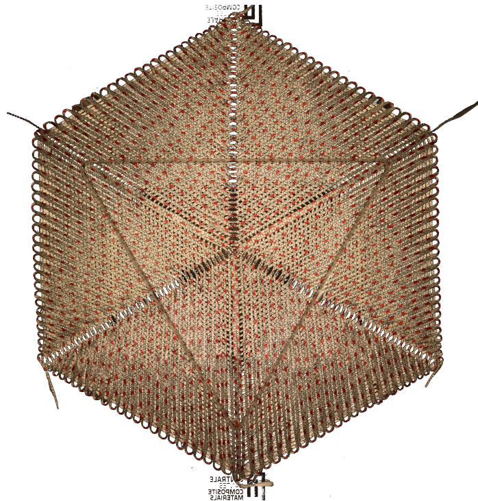
Figure 3.14: TFP preform with red ink markers drawn manually
