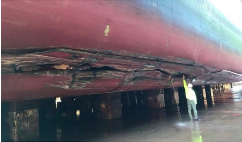
Figure 2.2: Seatruck performance grounding damage - From [21]
