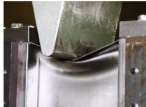
Figure 4.15: Web crushing from Zhang [37]
