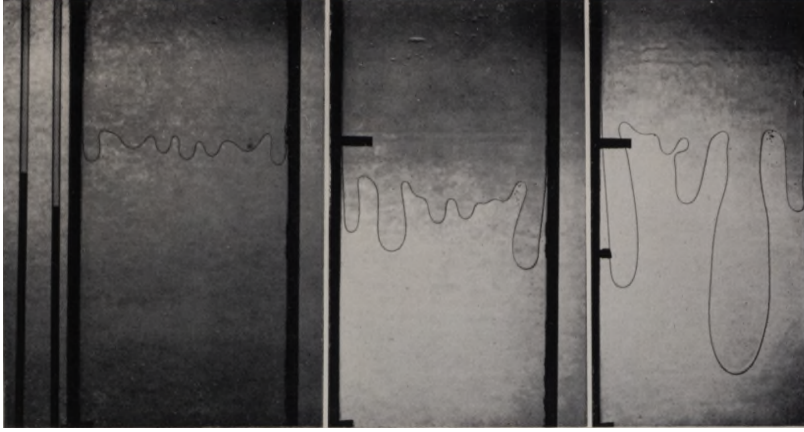
Figure 2.2: The celebrated “Saffman-Taylor” fingering observed at the interface between air (top) and glycerine (bottom), showing the development of instabilities and the inhibiting effect that the fastest growing finger has on its neighbors (SAFFMAN AND TAYLOR, 1958). In the first image, the velocity of the interface was V = 0.1 \text{ cm} \cdot \text{s}^{-1} and the critical wave length is \ell_{cr} = 1.2 \text{ cm} . The average wave length of the disturbance observed at initiation was 2.2 \text{ cm} which is in the expected range. Note that this experiment was done with the motion of the interface along the direction of gravity.
