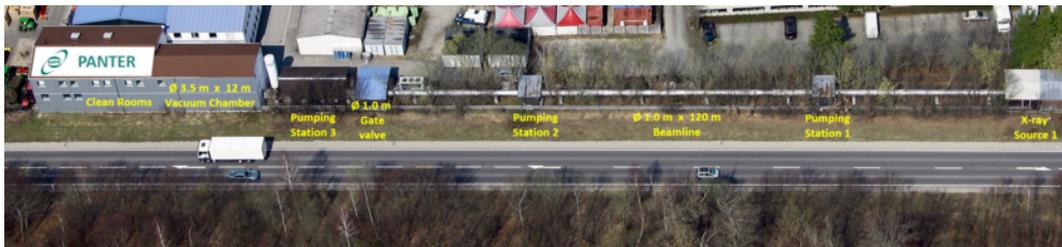
Figure 3.23: The panter X-ray test facility of MPE in Germany. The photo shows the vacuum tube of 130 m long and a diameter of 1 m, with the X-ray source system at one end and the test chamber at the other end. Credit: MPE
