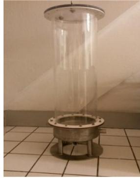
Figure 2.22: A 15 L photobioreactor with cylindrical main chamber.
