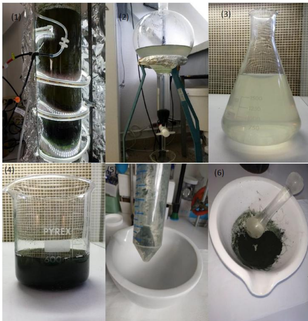
Figure 3.2: (1) The culture of Nostoc sp. ATCC 53789 is collected from the PBR (2) then it is added in a decantation flask for the first separation of the medium from the biomass (3) the medium after the decantation flask is disposed (4) and the wet biomass after the decantation flask is collected (5) that dry biomass is lyophilized to obtain dry biomass (6) and at last that dry biomass is pulverized with mortar and pestle
