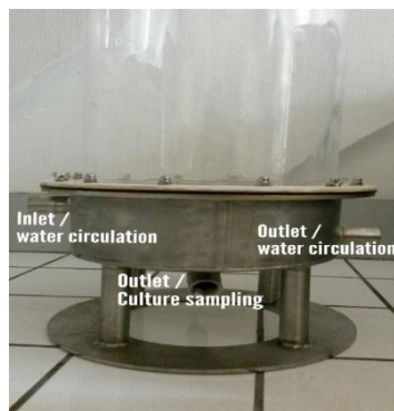
Figure 2.23: A metal jacket with water circulation system lays on the bottom of the photobioreactor.
