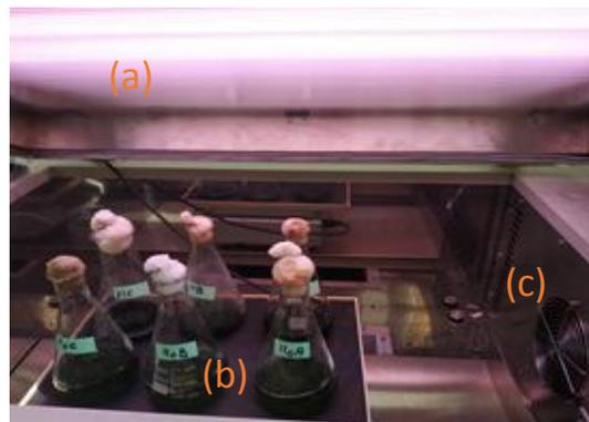
Figure 2.14: Photoperiod experiment instrumentation on Brunswick Innova 4340. a) Light panel b) agitation table c) temperature regulation through air climatization
