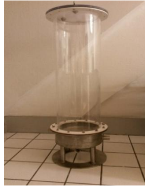
Figure 2.22: A 15 L photobioreactor with cylindrical main chamber.
