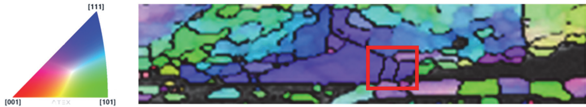
Figure 140: The orientation of the grain (along the x-direction) just at the healthy heel wire-metallization contact.
