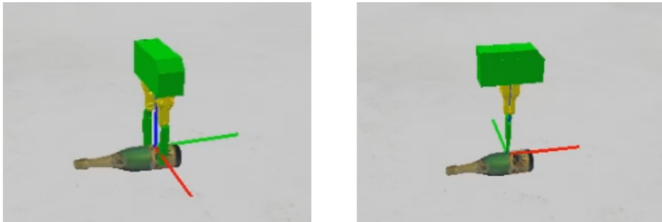
Figure 3.7: Simulation of two grasps inside the PyBullet environment. Left is a successful grasp, as the object will be lifted and correctly dropped away, right is a failed one
