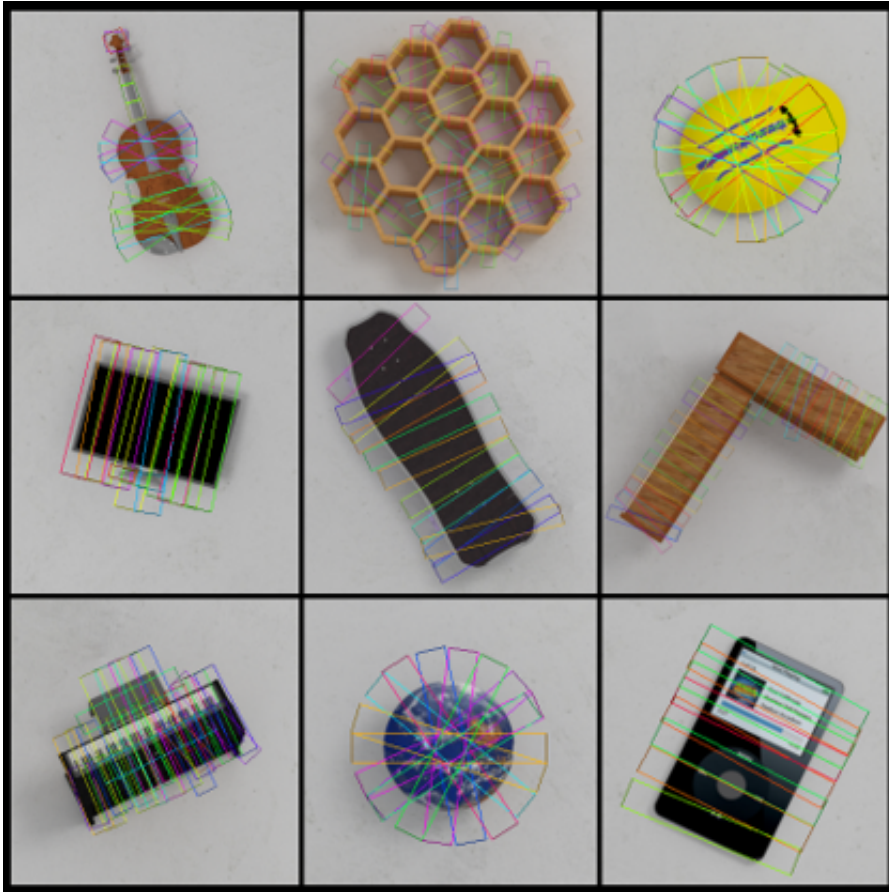
Figure 1.2: Examples of annotated synthetic images from our Jacquard Dataset. Rectangles represent successful parallel-jaw gripper locations.
