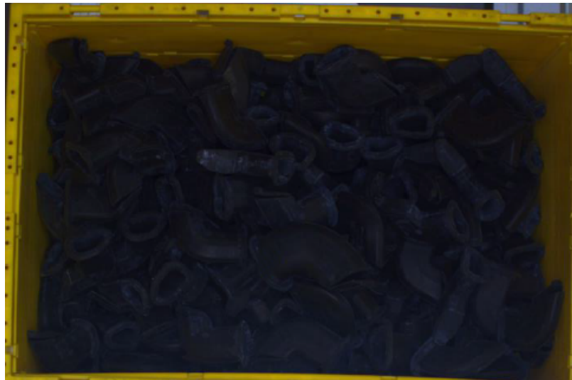
Figure 4.16: Example of a pile of textureless objects. An RGB image does not contain a lot of information to work on for this kind of industrial parts.
