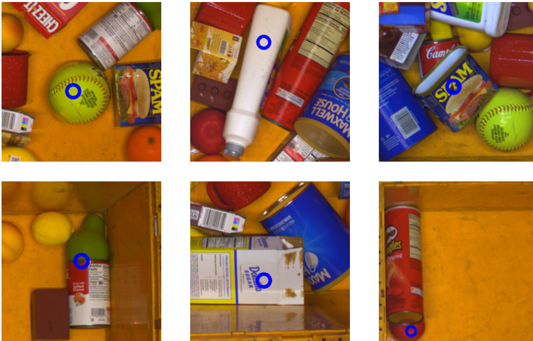
Figure 4.30: Close look at some grasps predicted by our network. Blue circle is the location of the suction cup. They are displayed over the RGB image for better visualisation. Some allow the network to successfully grasp the object (top row), while others fail at this task (bottom row).
