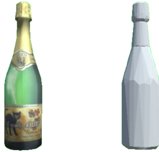
Figure 3.5: Visual comparison of an original model (left) and its three parts decomposed VHACD collision model (right).
