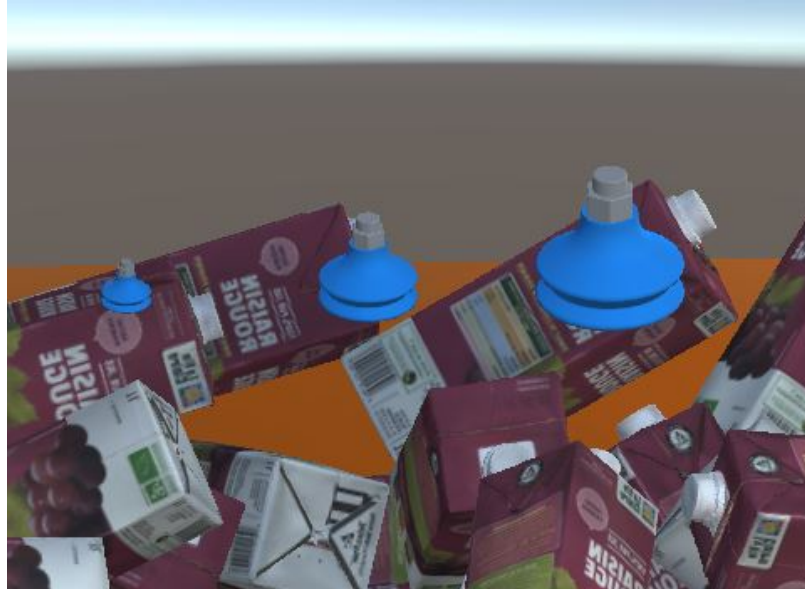
Figure 4.17: The three suction cups used to train the network in the context of a typical object pile in our simulation environment.
