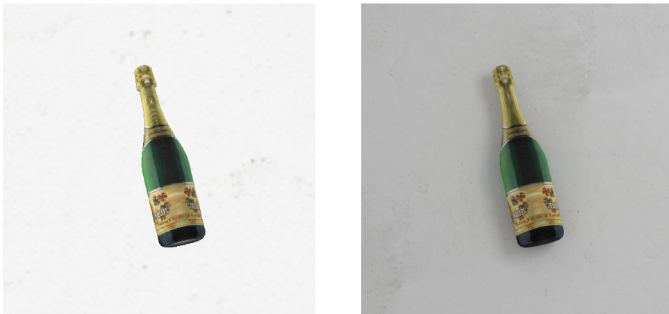
Figure 3.3: Comparison between the integrated Blender Renderer (left) and the ray-tracing Cycles Renderer (right).
