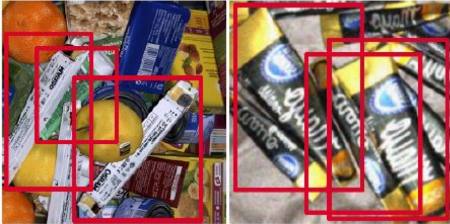
Figure 2.9: In object piles with many instances, a box detection algorithm is not sufficient to determine the location of objects. Multiple instances can lie inside each of the detected rectangles.
