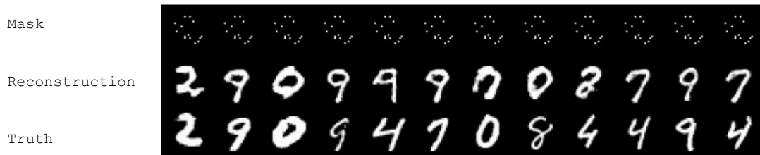
Figure F.4. – Samples of masks (first row), reconstruction (second row) and true data (last row) for Mnist dataset obtained using a cGAN approach following Isola et al. 2016, i.e including a \ell_1 +Gan loss as reconstruction objective for approximately 15 sampled pixels ( \lambda_s = 100 )
