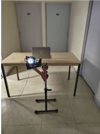
Figure 4.5 – Headlight of a vehicles used for data transmission
