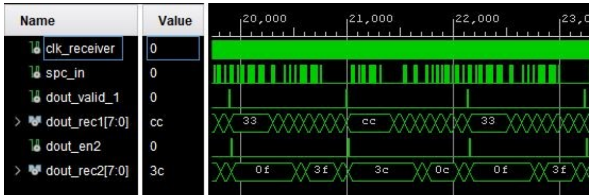
Figure 6.9: Recovered data from the two Tx's which are positioned at a distance of 20 cm from the Rx. The data were read through the built-in ILA of FPGA via a JTAG port.
