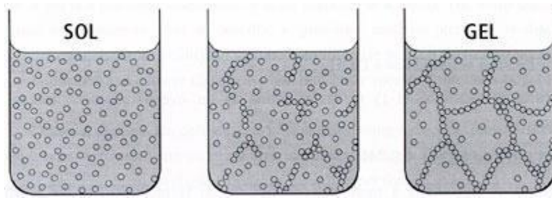
Figure 11 Behavior of the particles during the Sol-Gel process.
