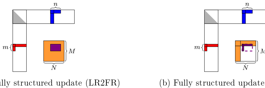
Figure 1.8: Representation of two different low-rank update options ( C \leftarrow AB ). Here, the contributing blocks A and B appear respectively in red and in blue. The updated block C is colored in orange and the impact of the contribution ( AB ) is in purple.
