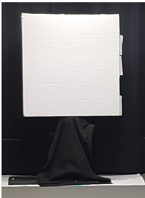
Figure 4.7: Wall target used for system calibration
