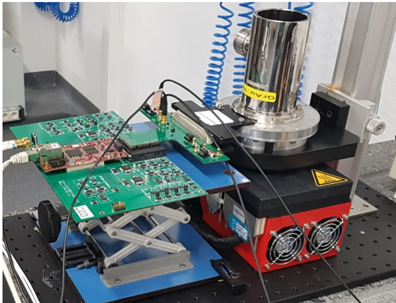
Figure 3.4: Testbench for the evaluation of the nonuniformity: the detector faces a blackbody emitting an uniform flux of photons.
