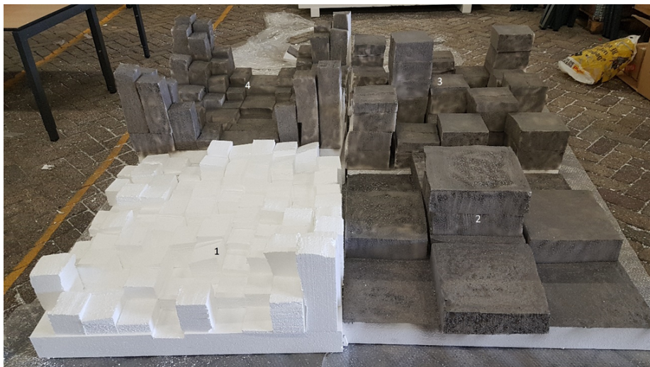
Figure 4.3: Polystyrene targets used to assess the system's resolution
