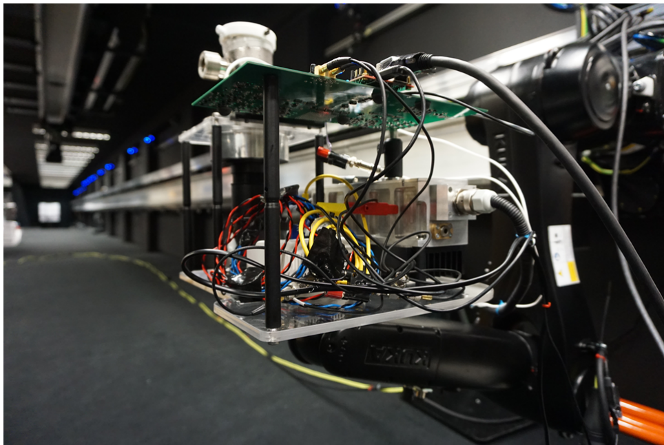
Figure 4.1: The Flash LiDAR is mounted onto the end effector of the robotic arm.
