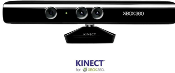
Figure 1.2: Example of a Projected-Light sensor: Kinect™ for XBOX 360.
