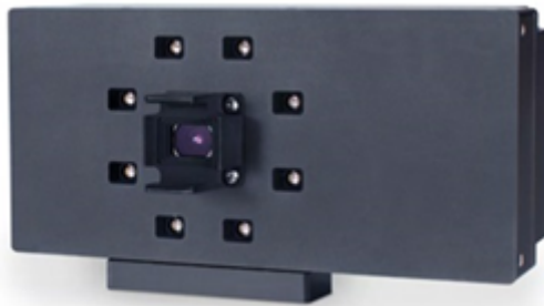
Figure 1.3: Example of a phase-based camera system: Basler's time-of-flight camera.
