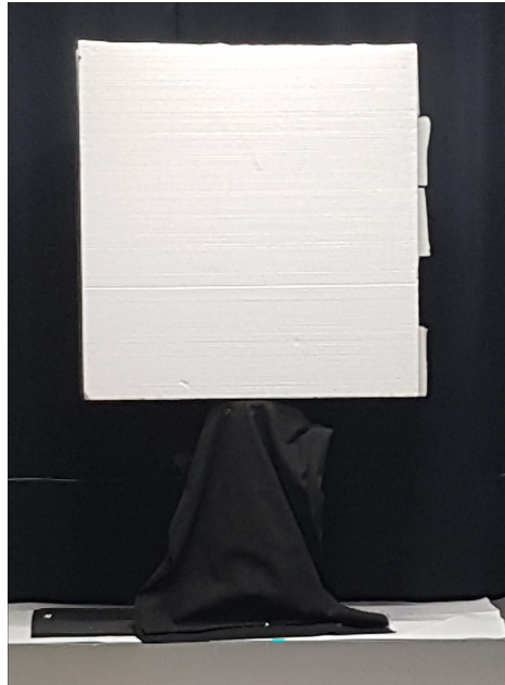
Figure 4.7: Wall target used for system calibration
