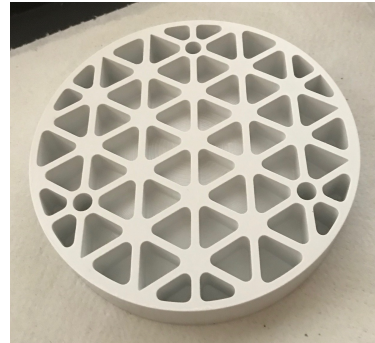
Figure 4.24: Back of the unpolished M3 mirror.
