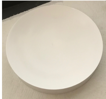
Figure 4.23: Front of the unpolished M3 mirror.
