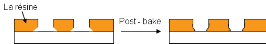
Figure III-22 - But du "traitement post-bake"
